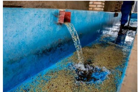
Image shows the beans passing through the floatation channels at Karambi coffee washing station
