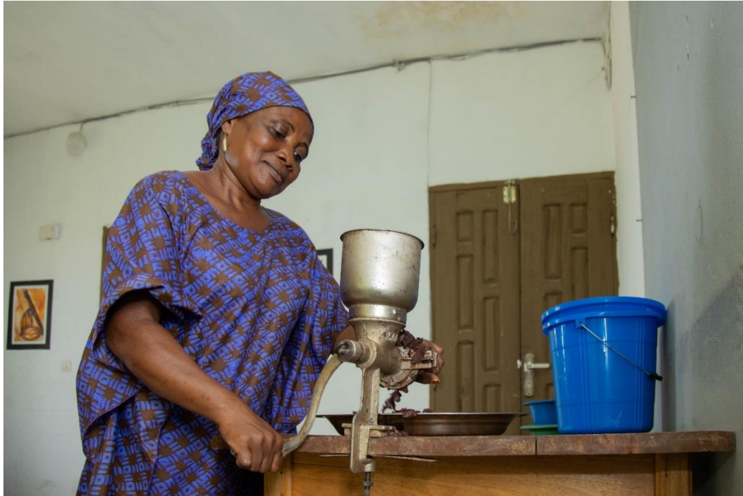
Juliette Assi Apo, member of CAYAT, grinding cocoa beans to produce powder to process into chocolate
